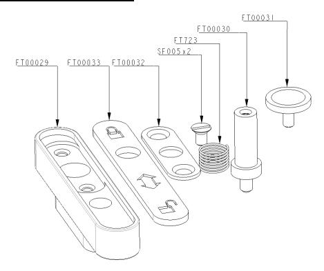
Upon receipt of the components, please check to make sure none are missing. The above image displays the components required to retro fit a single shootbolt assembly.
